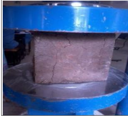
Fig. 8: Testing of Cube Specimen for Compressive Strength
