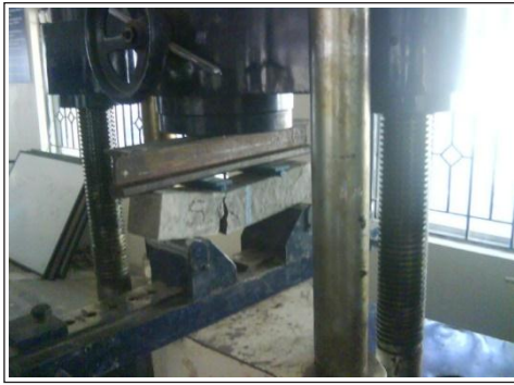
Fig. 10: Beam Specimen Subjected to Flexural Strength
