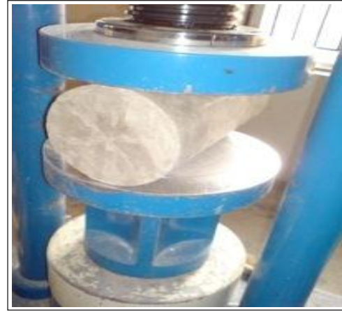
Fig. 9: Testing of Cylindrical Specimen for Split Tensile Strength
