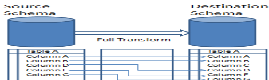
Figure 3. Conceptual overview – The full transform method
