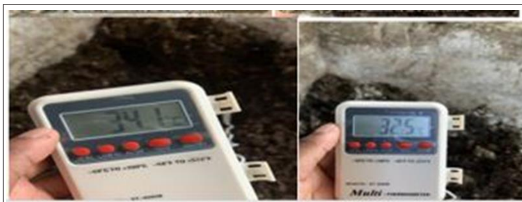
Fig. 2: Regular Temperature Detection via Probe Digital Thermometer
