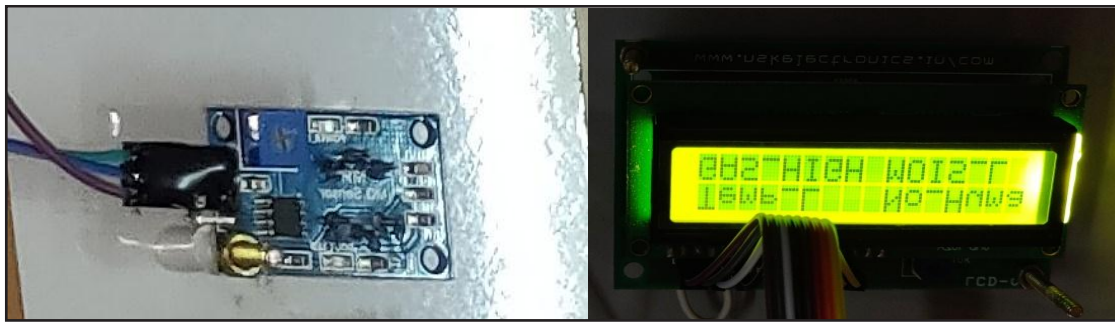
Fig. 5: Gas Level is High and Display Output as High
