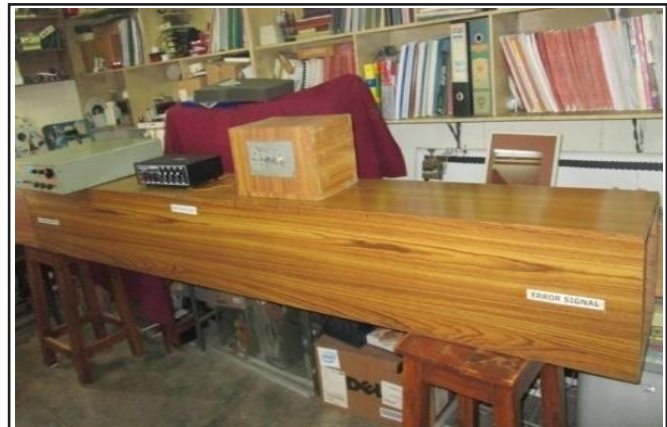
Fig. 6: Experimental Setup for Testing Analog ANCS with Speaker
