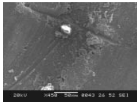
Figure 3 : SEM photograph at moderate operational conditions of load 49.05 N, sliding speed 1 m/s & temperature 400oC Three body abrasive
