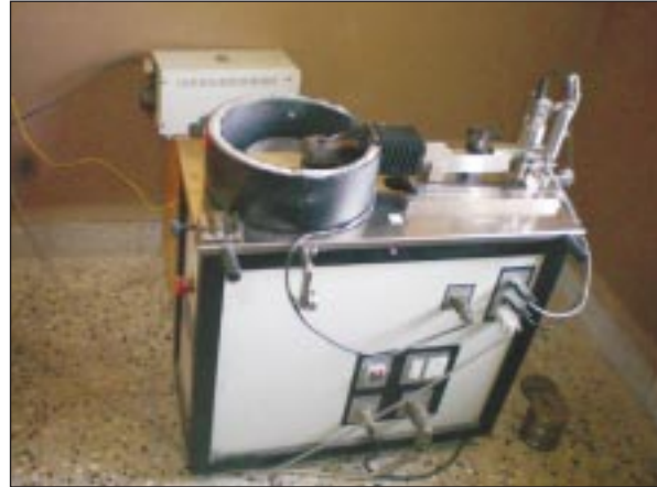
Figure 1 : Photographic view of high temperature wear-testing machine
