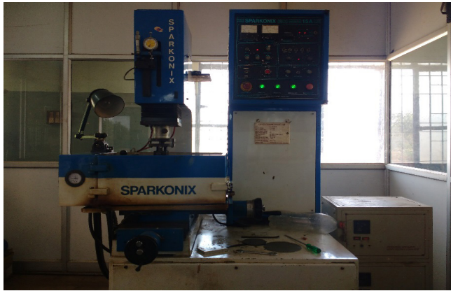
Fig. 1: Experimental Setup of SPARKONIX S50 EDM
