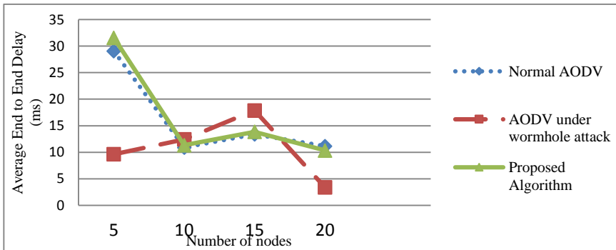
Fig. 5 E2E delay Vs Number of nodes with 2 wormhole nodes
