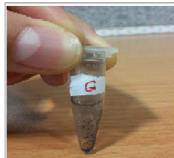
Fig. 7: Graphene Solution at Concentration of 0.5 Milligrams Per Milliliter of (Graphene in the Water Solvent as Stable)
