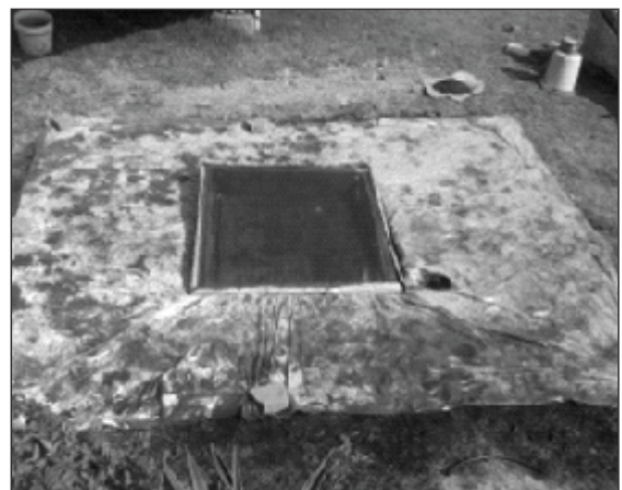
Figure 6: Photograph of solar still-3 (S-3) with blackened top surface and covered with polythene around it.
