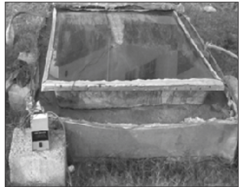
Figure 5: Photograph of solar Still-2 (S-2) without polythene.
