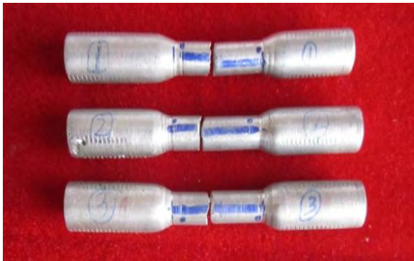
Fig. 4: ASTM sized tensile test work piece
