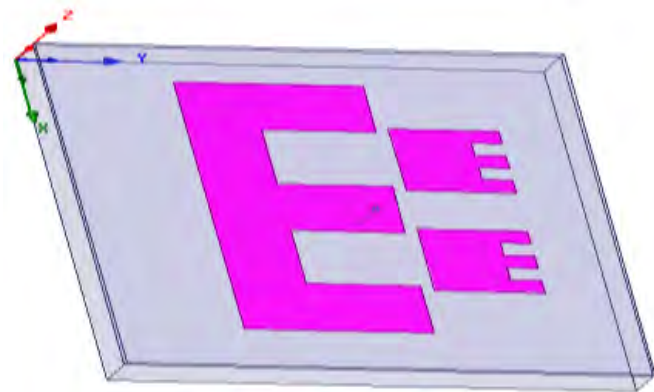
Fig. 5: E-Shaped patch antenna when the switch is ON
