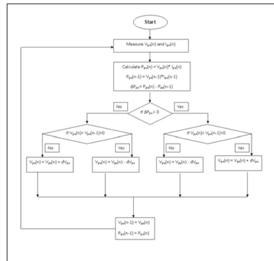
Fig. 2: Flow Chart for P&O Technique
