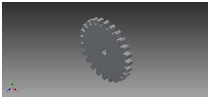
Fig. 2. 3D Modeling of Spur Gear in Autodesk Inventor 2014
