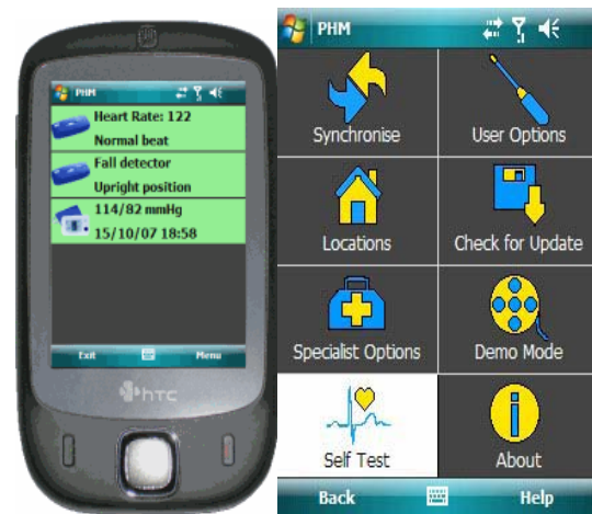
Fig. 2. PHM monitor and the self-test integrated into the PHM application.
