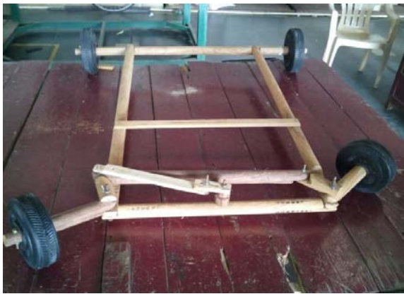
Figure 12: Prototype for Optimum Inner Steering Angle (54 degree), W/WB =0.58
