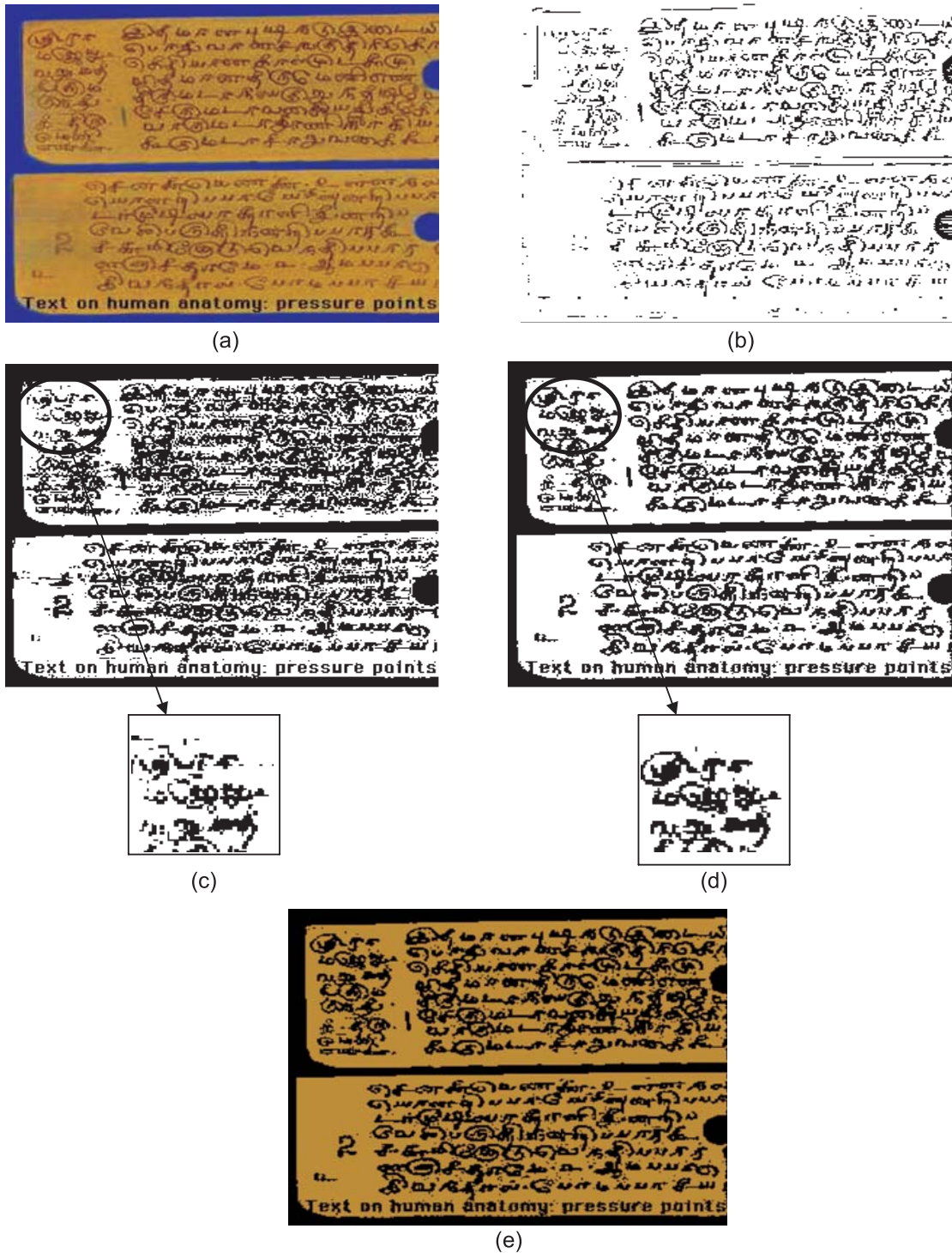
(a) Original image (b) Laplacian Sign technique (c) Otsu technique (d) Proposed technique (e) Color Image output with synthetic background.
